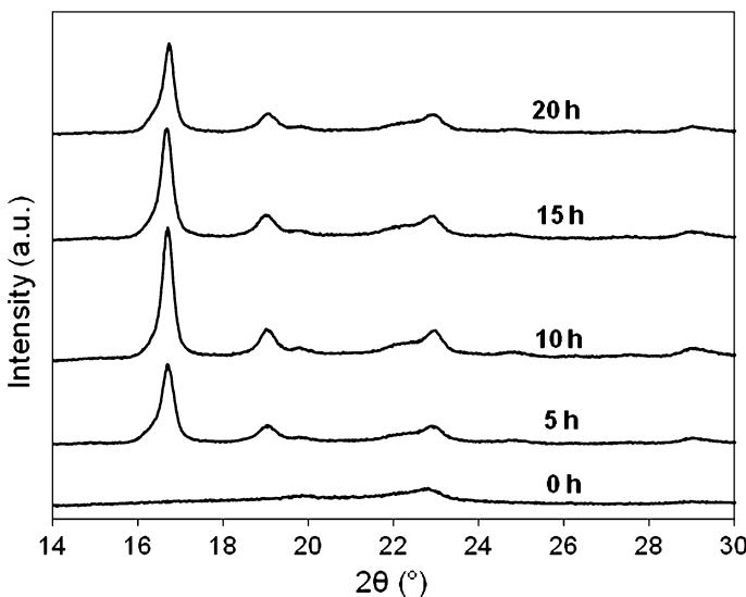
**Fig. 13** XRD patterns of 75/25 blend with different annealing time
