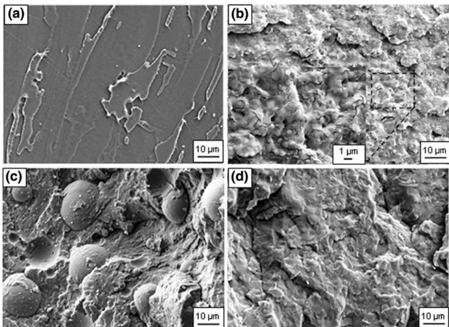
**Fig. 9** FESEM images showing the fracture surface of **a** neat PLLA, **b** 75/25 blend, **c** 25/75 blend, and **d** neat PBSL
