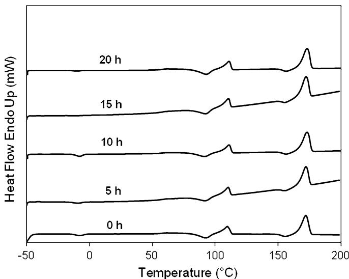
**Fig. 10** DSC thermograms of 75/25 blend annealed at 100 °C for various time periods
