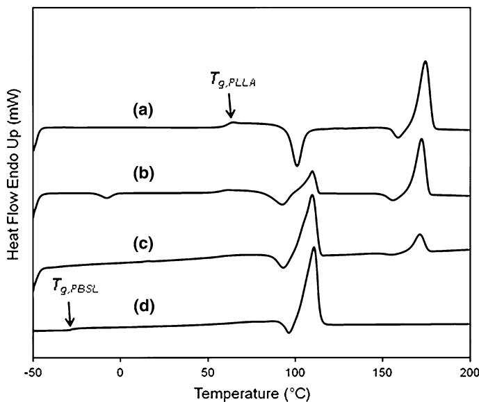
**Fig. 1** DSC thermograms of **a** neat PLLA, **b** 75/25 PLLA/PBSL blend, **c** 25/75 PLLA/PBSL blend, and **d** neat PBSL
